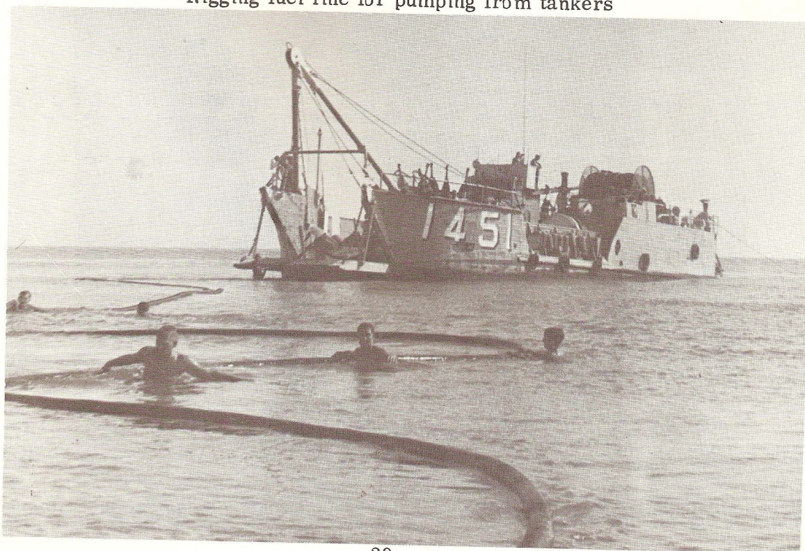
Rigging fuel line for pumping from tankers
