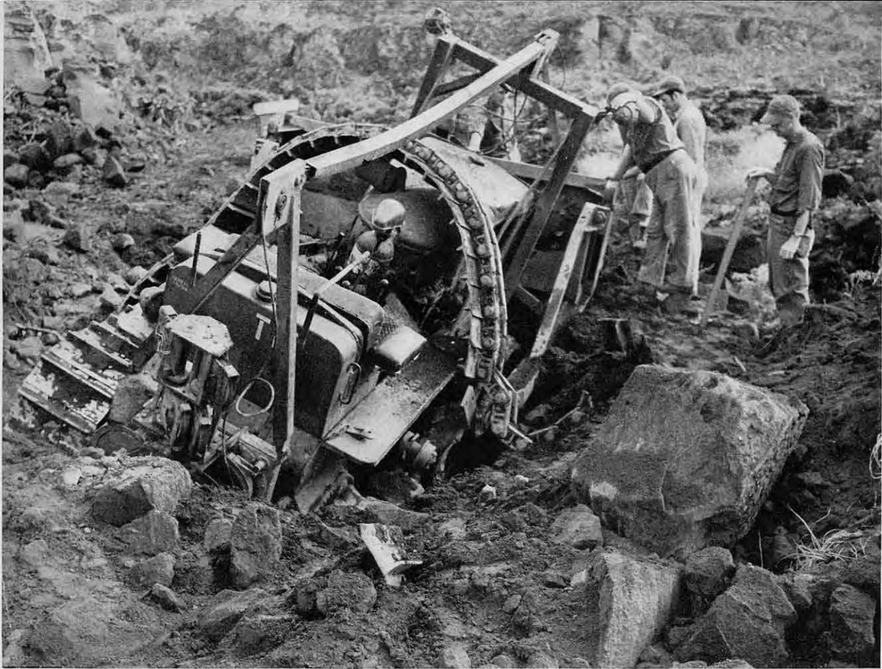
Another of the 95th's dozers that struck a land mine and was severely damaged. The operator, F. H. Krause escaped serious injury.
