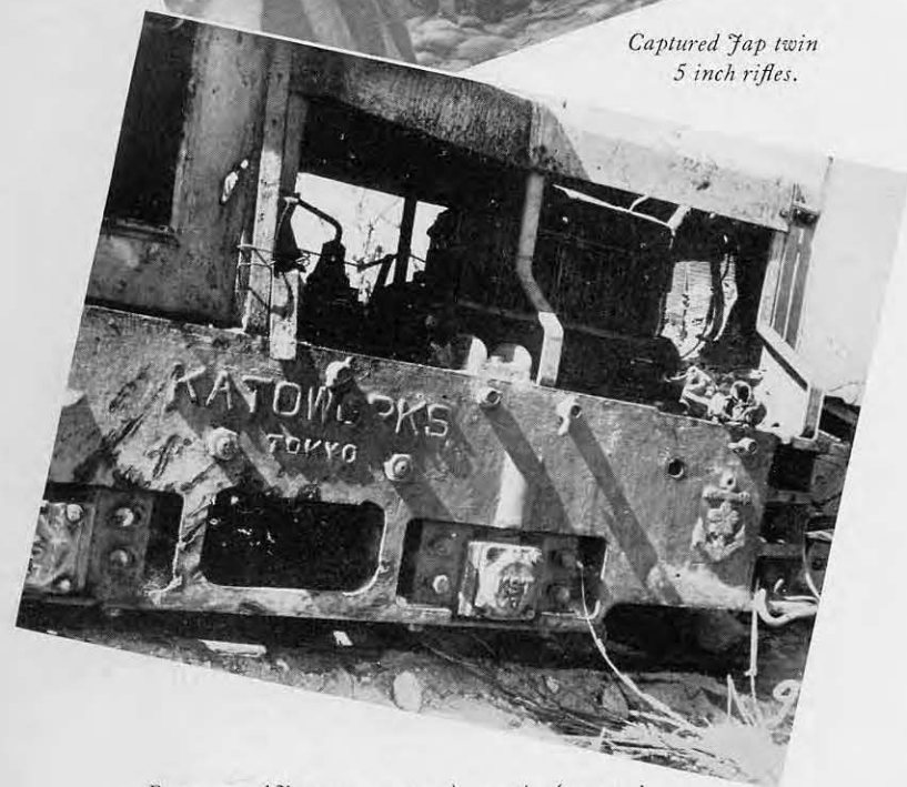
Remnants of Jap narrow-gage locomotive (powered with Chevrolet motor) note symbol of Japanese Imperial Marines.
