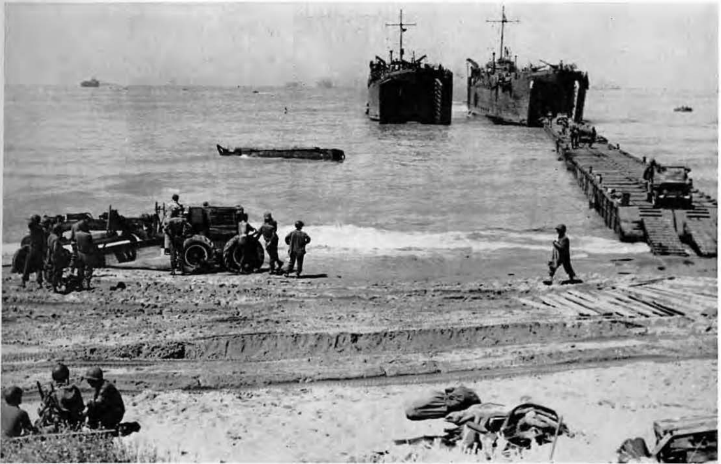
Bringing the war to the Italians, LST formed a large part of the huge armada that landed men and supplies on the shores of Sicily. Jeeps roll from one craft as another stands by, jaws open, ready to unload. Notice the pontoon causeway over which the jeep comes ashore.
