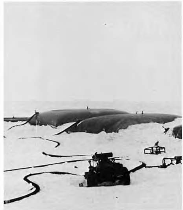
The manifold is connected to the fuel pump . . . and the fuel pump is connected to the fuel bladder.
