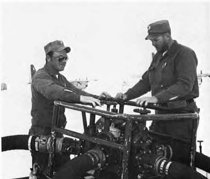
The fuel line is connected to the manifold (adjusted by ABF3 James Fjora, Jr., left, and ABF2 Donald Richardson, right . . .
