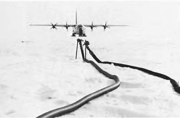
The plane is connected to the fuel line . . .
