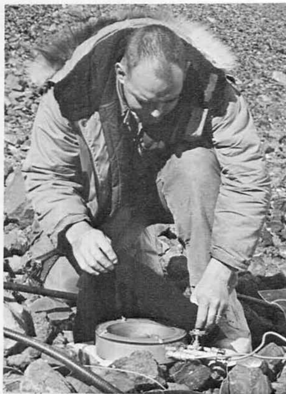
Ted Gannutz, USARP, Clark University, conducts lichen photosynthesis experiments with the aid of a respiration chamber.
