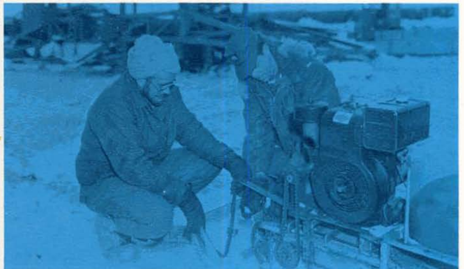
BELOW - EOC Harry M. Armagost, left, and LTJG Michael A. Merback discuss a slight problem with the chain drive of a motor toboggan. In the background is a snow planer used in resurfacing the landing area at Williams Field.
