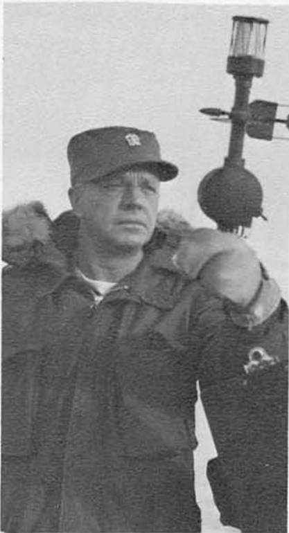
Lcdr Vincent Law takes wind velocity and direction readings with a hand held anemometer.
