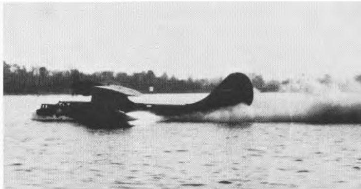
Truax and his staff are shown at left during a visit from Dr. Van Karman (in white coat) of Cal Tech. Above, JATO units light off during 1942 PBV tests in Severn River. Craft made one successful takeoff prior to mishap.
