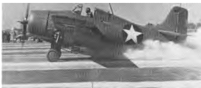
Asphalt potassium perchlorate JATO was demonstrated in 1943 on F4F-3.
