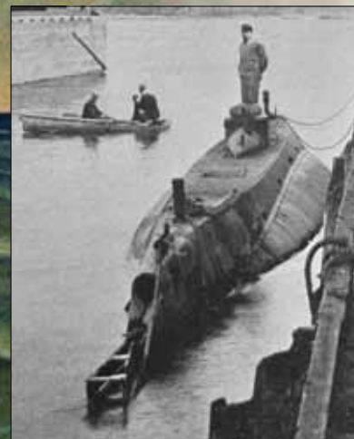
Holland VI's aft dynamite gun is visible at the submarine's stern, both in this 1898 photograph and in the Koerner & Hayes lithograph made at about the same time. (HRNM Collection/Library of Congress)
