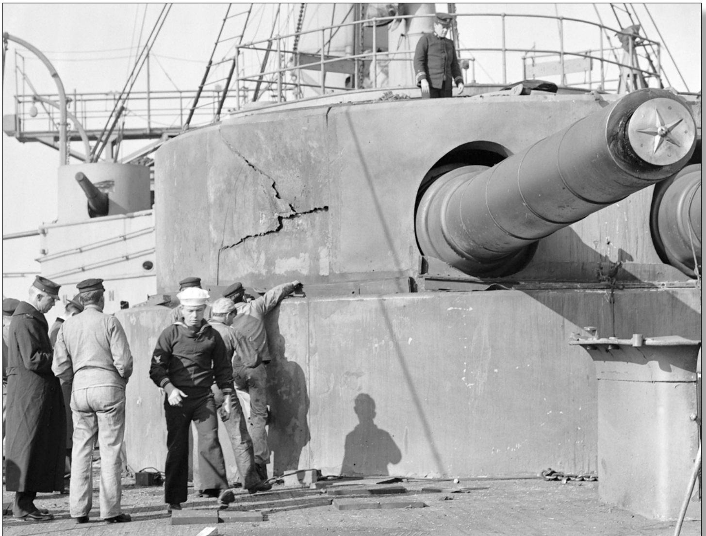
A photograph taken after the first Thorite detonation shows the large crack in the armor on the port side of Puritan's aft turret, where it was pushed in approximately 8 inches. Animals reportedly brought by Willard Isham and placed in crew positions within the turret, however, were uninjured. (Courtesy the Library of Virginia)
