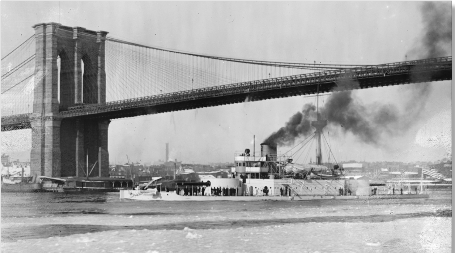
USS Puritan makes her way under the Brooklyn Bridge, through the icy East River, presumably not long after her commissioning on December 10, 1896. With a length of 289 feet, 6 inches, a beam of 60 feet, one inch, and a draught of 18 feet, USS Puritan was extensively modified during her over two decades of construction and development, looking like the missing link between a monitor and a battleship by the time she was finally completed. (Library of Congress)
