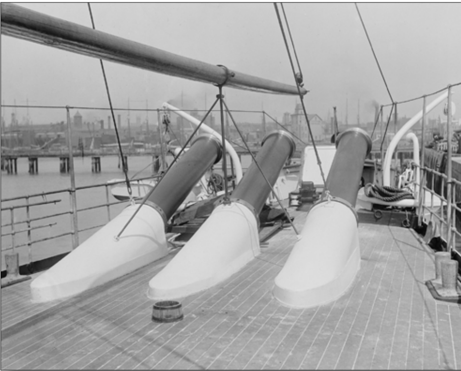
Although the ends of the three smooth-bore guns only protruded about 7 feet above the forecastle at a fixed 18-degree angle, they belied the colossal 55-foot length of the barrels, which went two decks down. (Detroit Photographic Co. Collection, Library of Congress)
