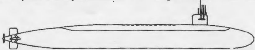
Measuring over 557 feet in length and displacing 18,750 tons, the Ohio -class ballistic missile submarines are the largest American submarines ever built and the second largest in the world. They have the reputation of being among the most quiet naval vessels in service. Each of these silent giants carries 24 Trident ballistic missiles while performing its strategic nuclear deterrent mission.
