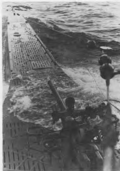
This is a picture of a Type VII U-Boat which was the mainstay of the Kriegsmarine's submarine force during World War II. Between five to eight of these boats operated in American waters in 1942. Displacing 769 tons, it was capable of 17 knots on the surface and 7 1/2 knots submerged. (National Archives photo)
