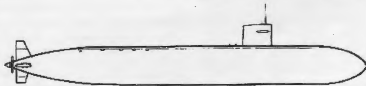
With 61 boats built, the Los Angeles -class is the most successful submarine design of the post-World War II Navy. It measures over 360 feet and displaces around 7,000 tons. Twenty-five of these boats are based at the Norfolk Naval Station. The class has since undergone two improvement stages. Starting with USS Providence (SSN-719), the Los Angeles -class was equipped with Tomahawk cruise missiles. In 1988, the Navy commissioned USS San Juan (SSN-751) which became the first attack submarine to be equipped with a vertical launch system (VLS). In addition to the VLS, the bow planes were taken off the conning tower and moved to the front of the boat.
