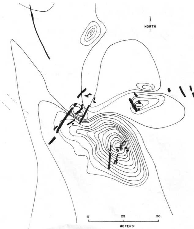
This is a diagram showing the results from a 1987 magnetic survey of Cumberland. The dark black lines represent magnetic contacts (Cumberland's hull is in the center) and the thinner line represents the contour of the floor of the James River. (U.S. Navy photo)
