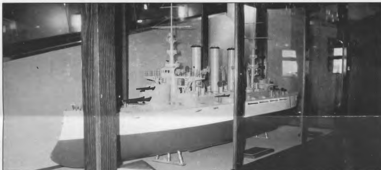
The beautiful Virginia model is painted in the standard "Great White Fleet" colors consisting of a red underwater hull, a brilliant white upper hull, a panama buff superstructure, stacks and turrets, purple/brown gun barrels and sanded pine decks. The model is made of wood (mostly pine) and brass. (Photo by Marta Nelson)
