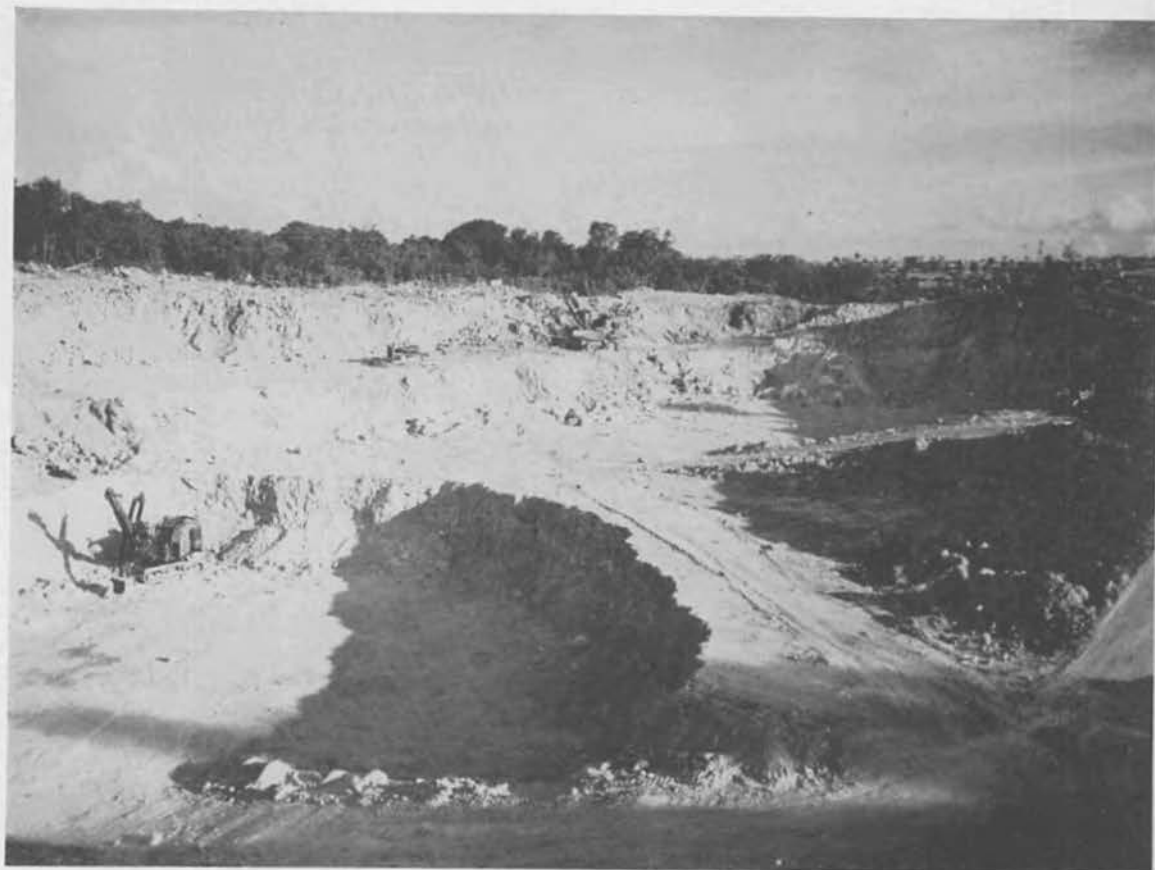
Three tier operation in Quarry.
