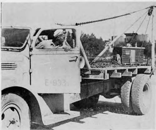
E. F. Deacon, MM2c, on this winch truck prepares to pick up and move a heavy piece of machinery.
