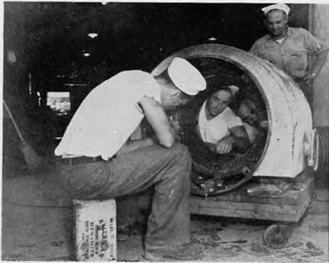
Repairing this 125 h.p. electric motor presented quite a problem to the men of the motor repair shop especially since there was no wire of the correct size available to wind the necessary coils. They weren't stopped for long, however, and by improvising and substituting, and with several days and nights of hard work soon had the motor back into service. Show here are Electrician's Mates Ralph Guida, Jack Berner and F. G. Petzold.
