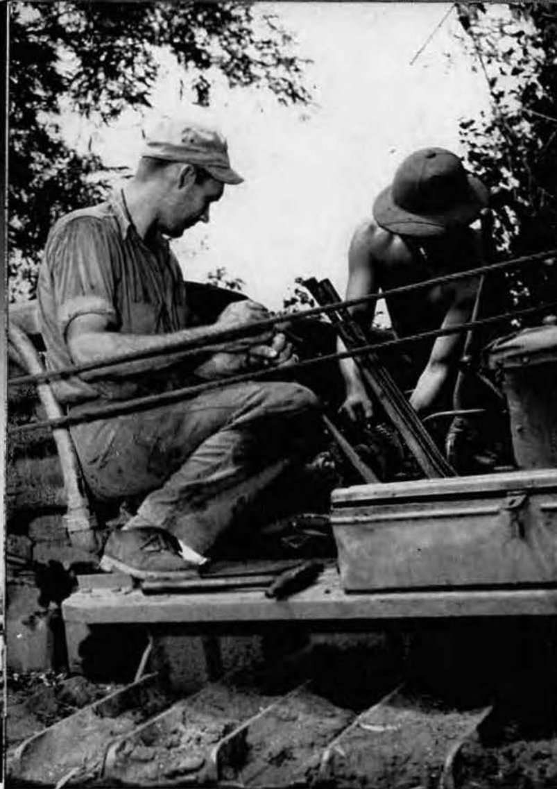
Mechanics adjust clutch on a huge caterpillar D-8 bulldozer.
