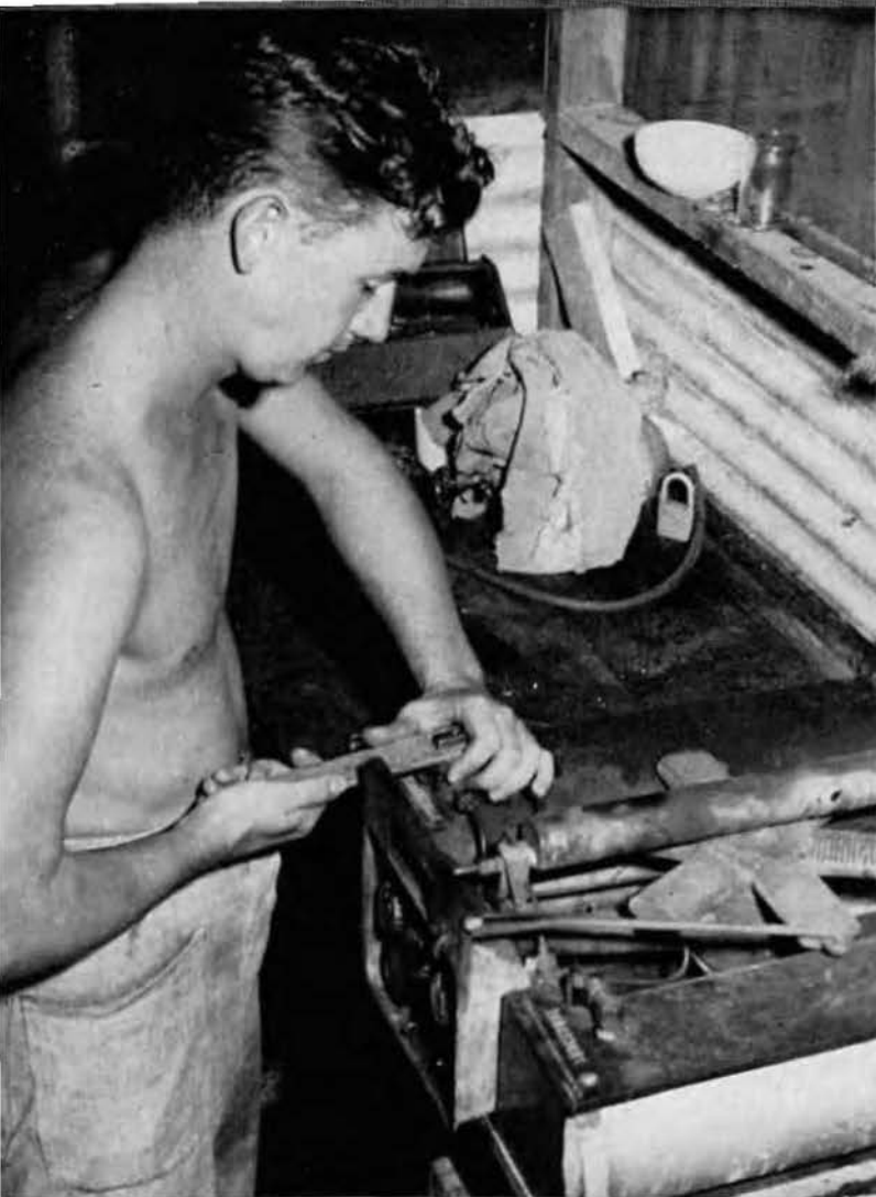
Stove repairman makes adjustment on field range.
