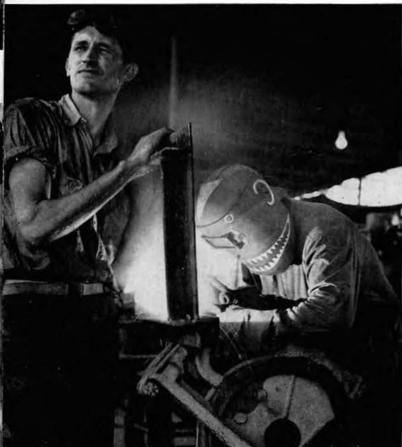
Lane and Sommers repair a Japanese anti-aircraft gun mount for use as a malaria control sprayer.
