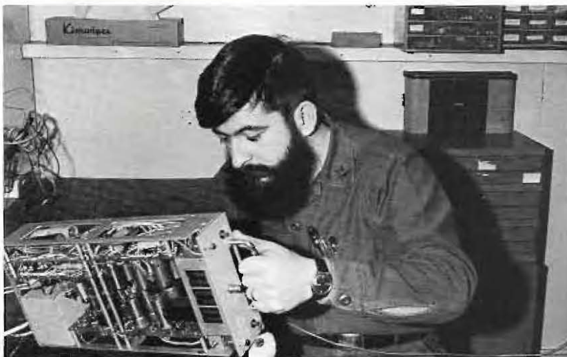
INSTRUMENT TECHNICIAN, Joe Marquez, performs preventative maintenance on the heart of a seventy-four point temperature scan (ABOVE) This is referred to by PM-3A as "open heart surgery". (AT
