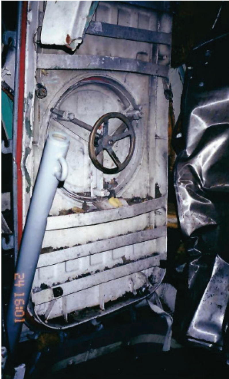
When the ship was hit, this watertight hatch was blown open and could not be closed again. (Courtesy of William Merchen)
