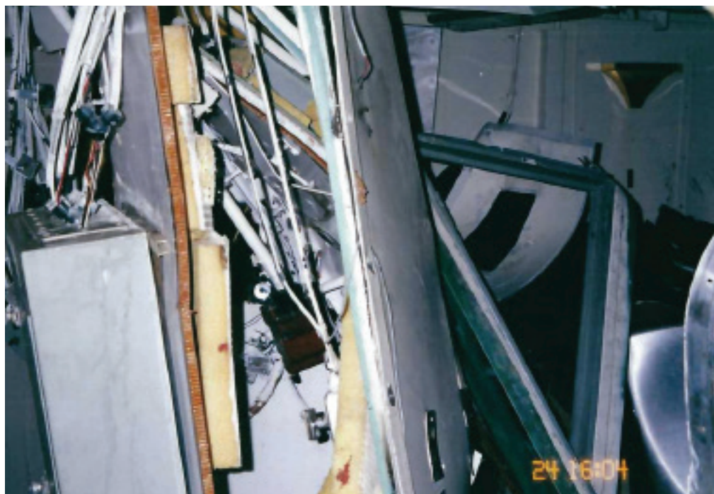
This image shows the false bulkhead that DC3 Merchen and his fellow shipmates ripped open to get to the Sailors trapped in the chief’s mess. (Courtesy of William Merchen)
