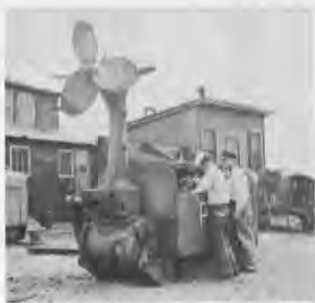
The ship repair unit may also service outboard propulsion units for pantoon structures.
