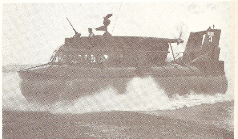
Patrol Air Cushion Vehicles (PACVs) were tested for use in both Market Time and Game Warden operations. Craft travel over a cushion of air.
