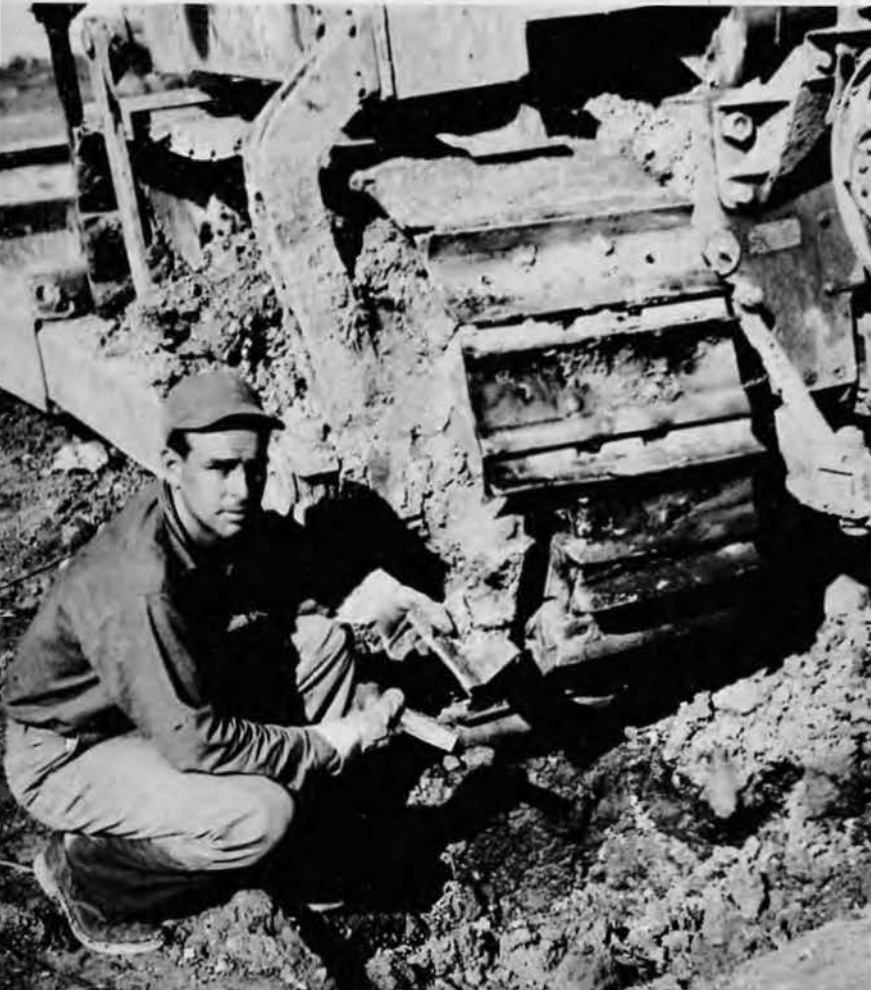
Fred W. Balke holds pieces of track from 'Dozer damaged by Jap land mine.
