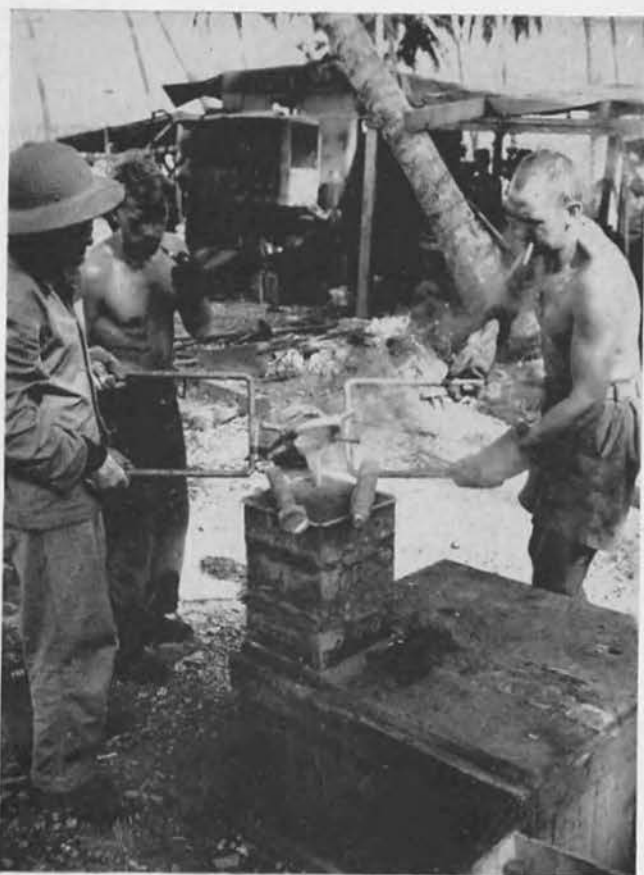
Salvaged Jap brass being molded into bushing stock at Guadalcanal by L. G. Domyan, Castle, Strzalkowski.
