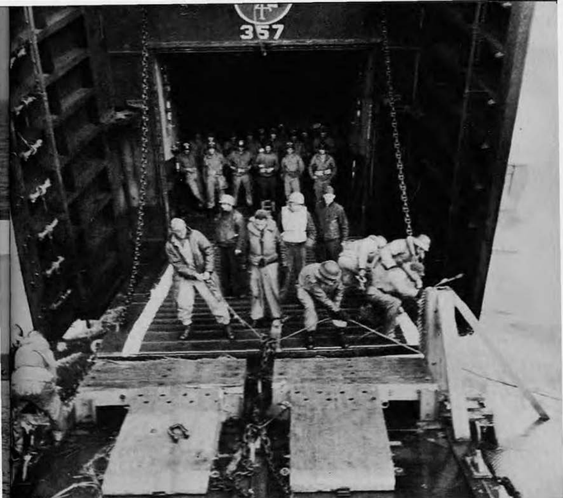
Marriage was made with great difficulty: Notice the port knee torn off
