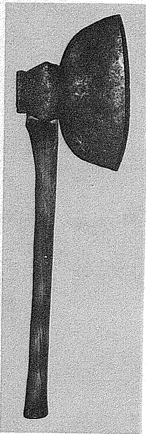
(Top) German style "goose-winged" broadax. (Left) American broadax with basiled or chisel-edged blade. (Right) American handax with chisel-edged blade. Some of the shape has been lost through years of resharpening.
