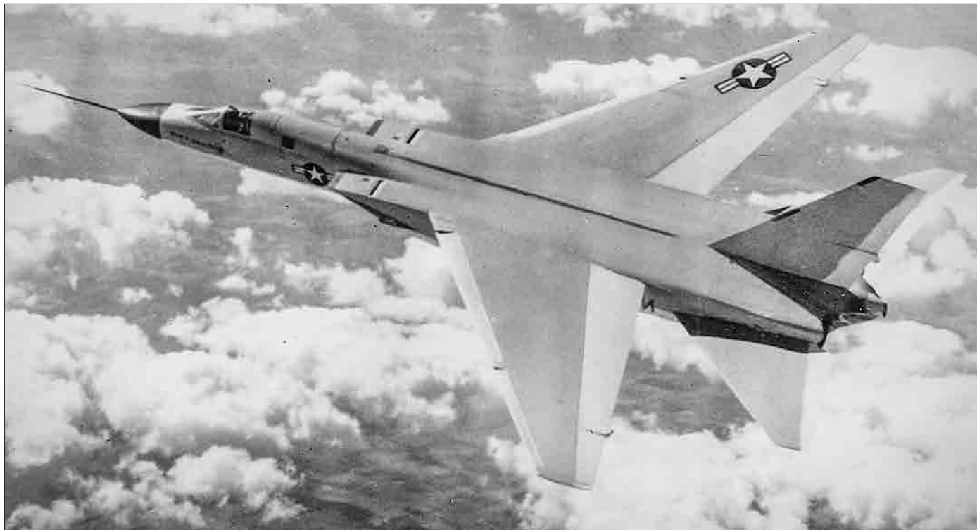
The A3J-1 Vigilante had a unique, but unsuccessful, bomb bay—a tunnel between the plane's twin engines from which the weapon attached to two expended fuel cans was ejected rearward. The type went on to become a successful supersonic reconnaissance aircraft.
