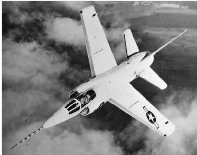
The supersonic F11F-1 Tiger had its origins in the subsonic F9F Panther and Cougar series of aircraft. This early prototype displays the plane's planform.
