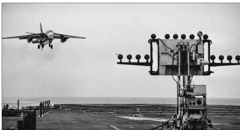
Equipment development encompasses all phases of naval aviation. An early mirror landing system aids an A3D Skywarrior as it lands on board an aircraft carrier.
