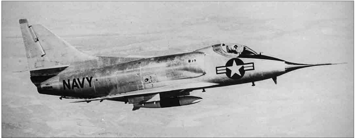
The seventh of nine YA4D-1 Skyhawk test aircraft, BuNo 137819, carries a Douglas NAVPAC (navigation package) during a trial flight, c. May 1956.
