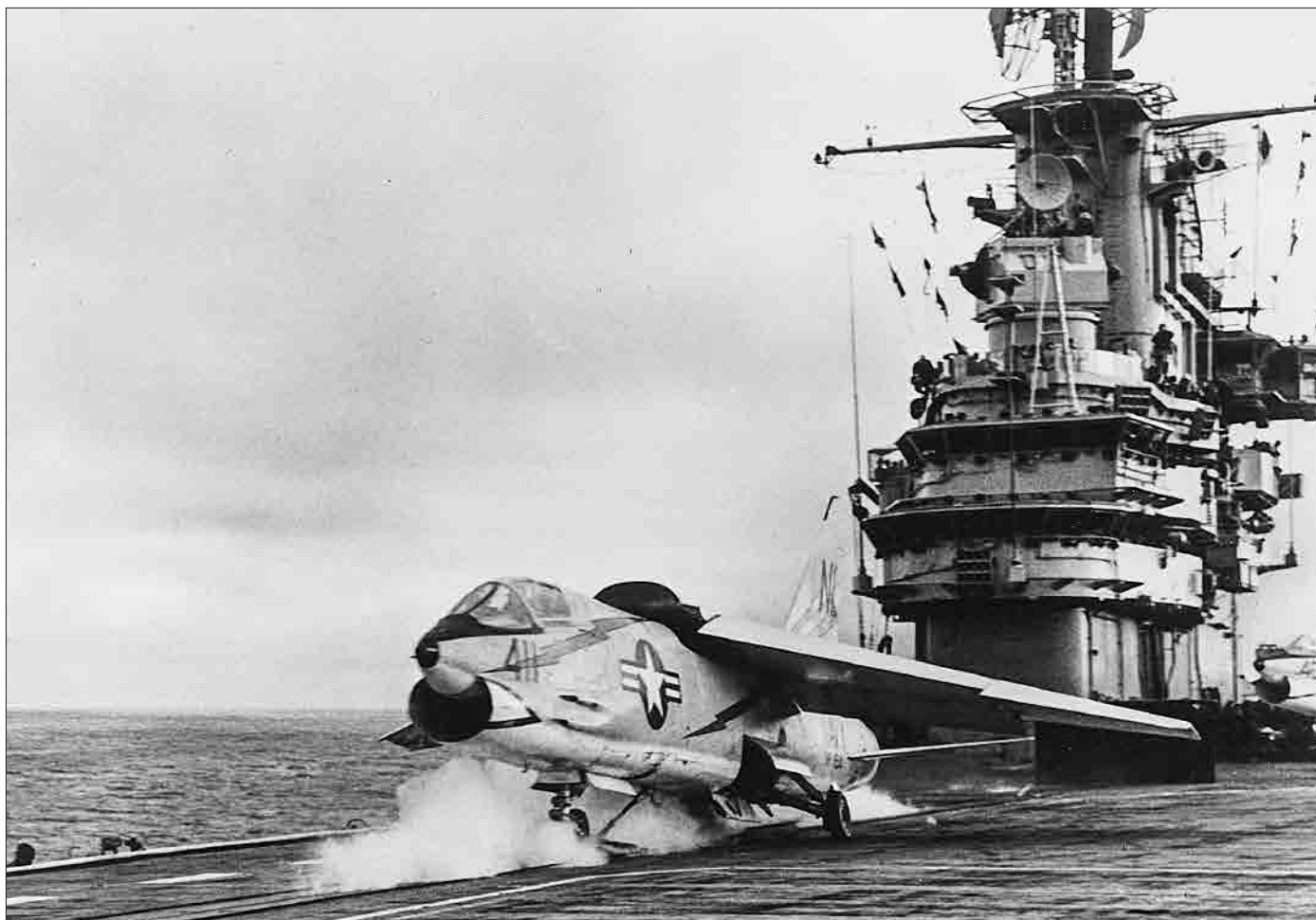
One of Hancock's (CVA 19) bow steam catapults launches an F8U-1 Crusader of VF-154 during carrier qualifications on 25 November 1957.
