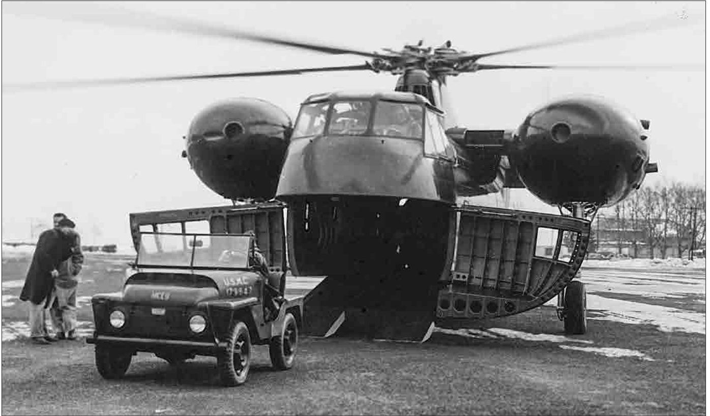
The Marines' HR2S-1 Mojave could carry 26 fully equipped troops or up to three jeeps, c. 1956.
