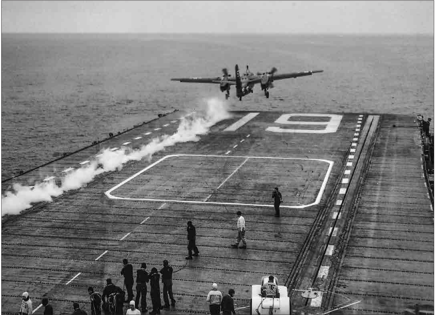
Cmdr. Henry J. Jackson pilots the first aircraft—an S2F-1 Tracker—to be launched by a steam catapult from an American carrier. The operational trials on board Hancock (CVA 19) took place on 1 June 1954.
