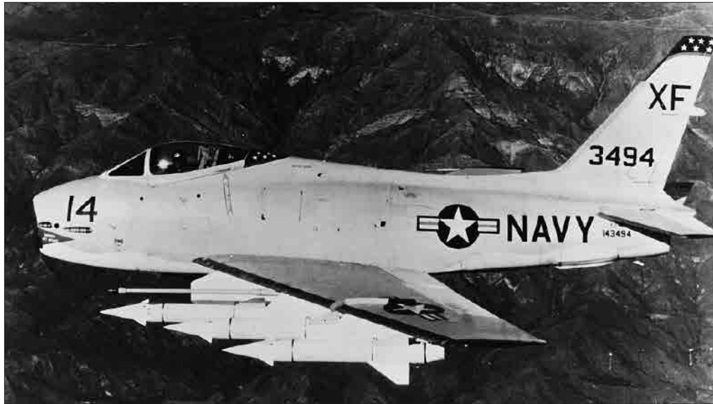
An FJ-4B Fury, BuNo 143494, of Air Development Squadron (VX) 4 carries a full load of five ASM-N-7 Bullpup air-to-ground missiles and their guidance pod, 16 April 1958.
