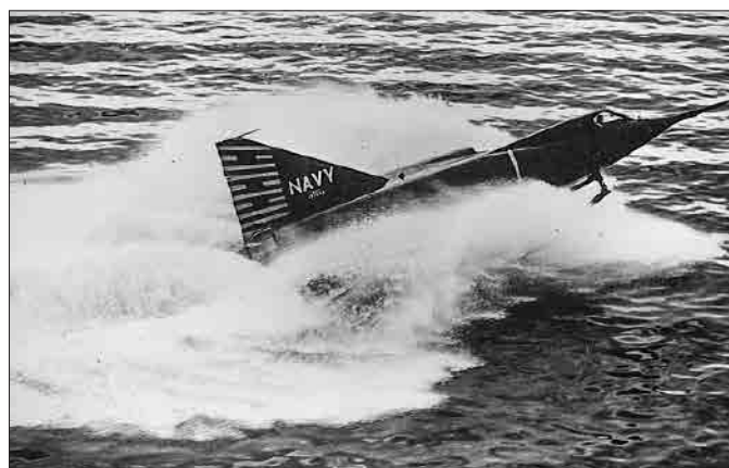
The XF2Y-1 Sea Dart hydro ski fighter throws up a massive wake during early taxi trials, which began in San Diego Bay in mid-December 1952.
