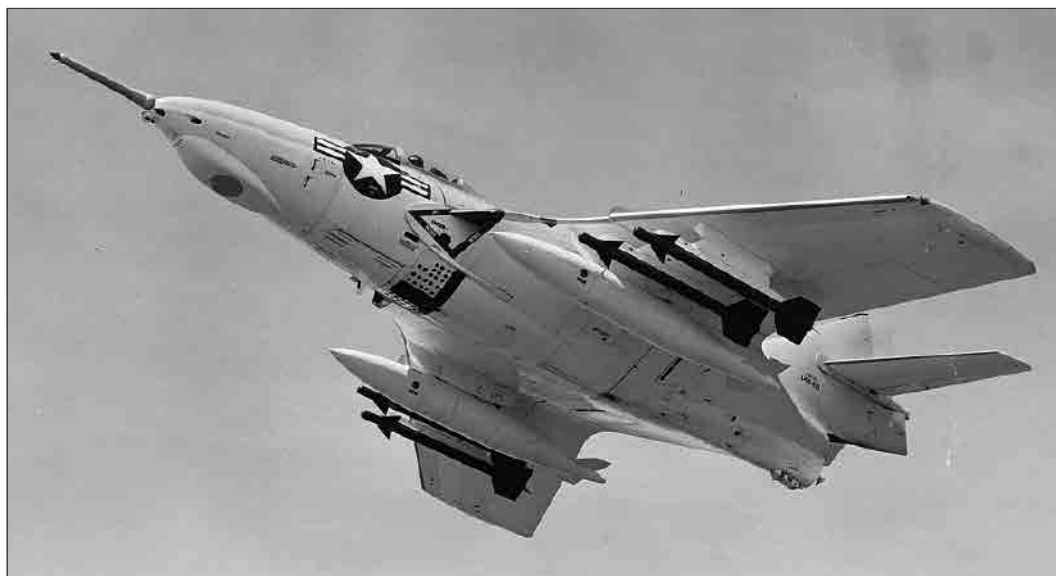
This F9F-8 Cougar, BuNo 141140, carries AAM-N-7 Sidewinder air-to-air missiles in addition to two auxiliary fuel tanks.
