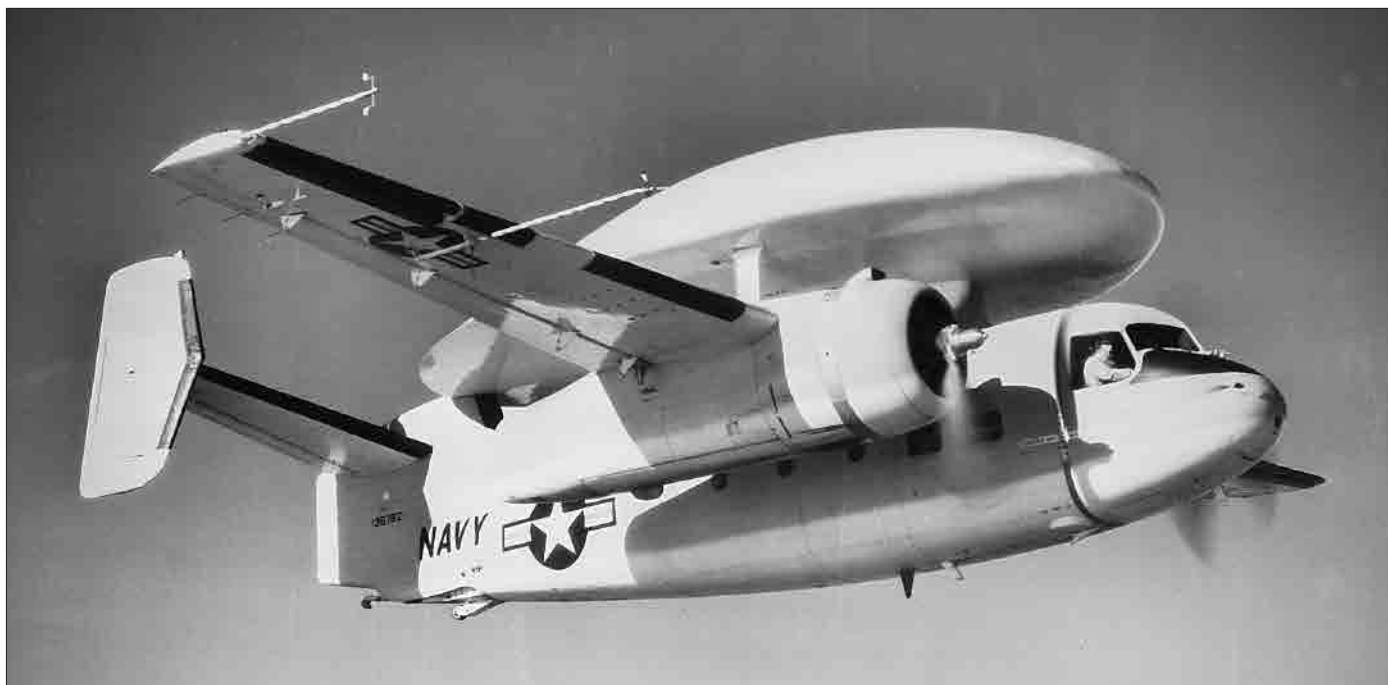
This TF-1 Trader, BuNo 136792, carrier onboard delivery transport has been converted into the aerodynamic prototype—without internal electronic systems—of the WF-2 Tracer carrier-based early warning aircraft.
