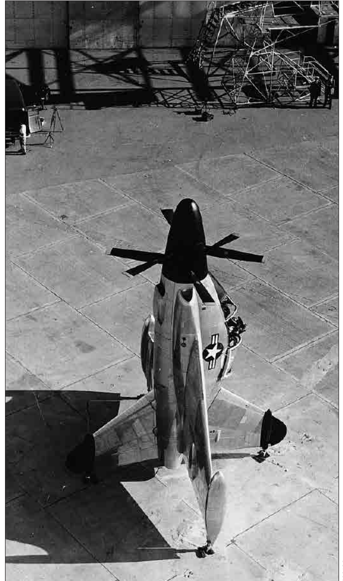
Only one of three XFY-1 experimental vertical takeoff fighter prototypes was completed and flown.
