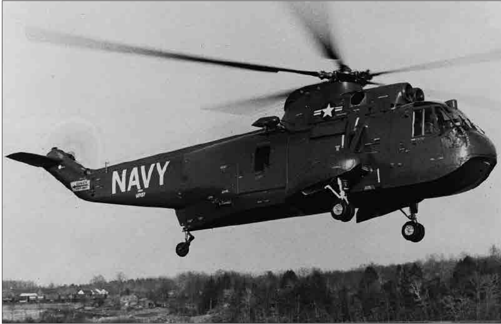
The first prototype HSS-2 Sea King, BuNo 147137, all-weather antisubmarine helicopter made its initial flight in March 1959.
