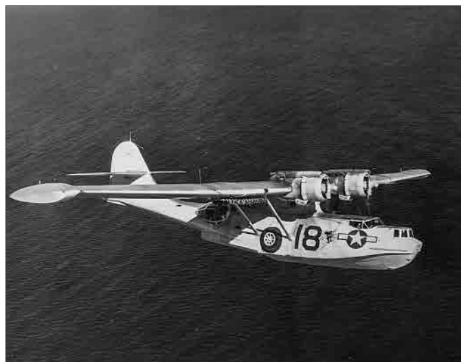
An amphibious PBY-5A Catalina of VP-63, based out of Port Lyautey, Morocco, carries antisubmarine retro-rockets while on patrol of the Strait of Gibraltar.
