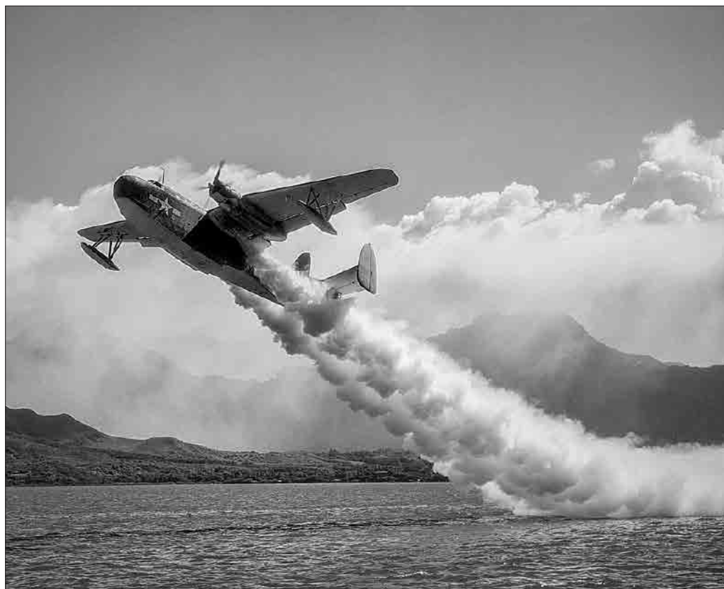
A PBM Mariner launches using jet-assisted takeoff (JATO) rockets.
