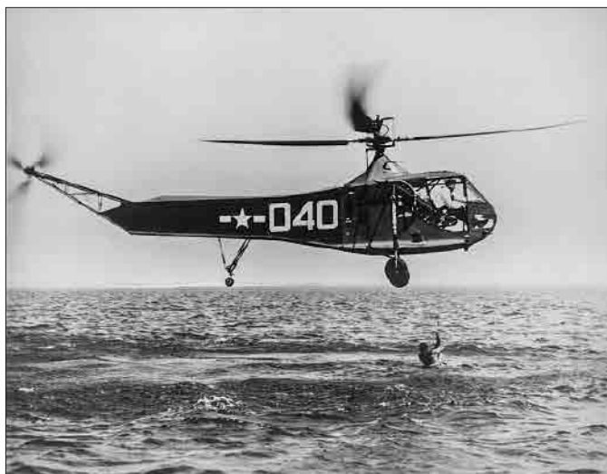
An HNS-1 Hoverfly, BuNo 39040—the Navy's first helicopter type—from Coast Guard Air Station Brooklyn, N.Y., demonstrates its search and rescue capabilities in Jamaica Bay on 25 August 1944.
