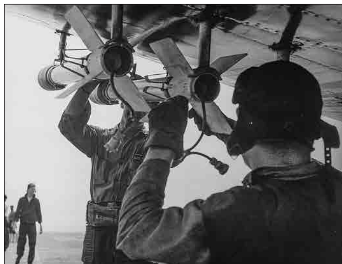
Aviation ordnancemen mount 4.5-inch high-velocity rockets onto a plane.
