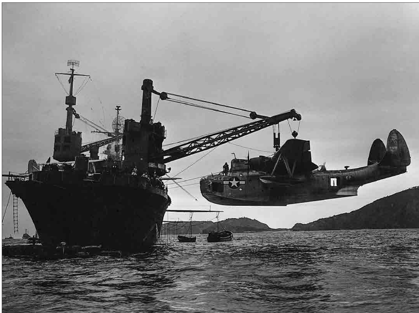
A tender hoists a PBM on board to service the Mariner.
