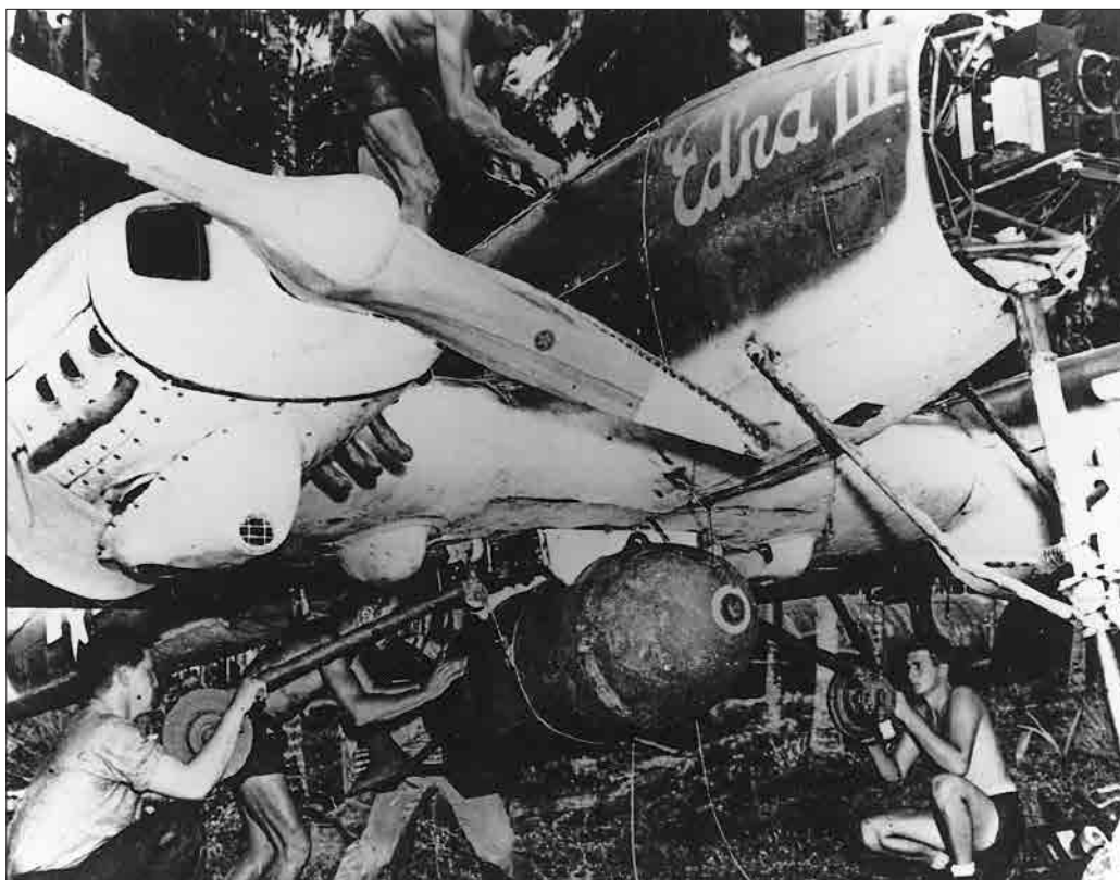
Sailors mount a 2,000-pound bomb on a TDR-1 assault drone in preparation for an attack.
