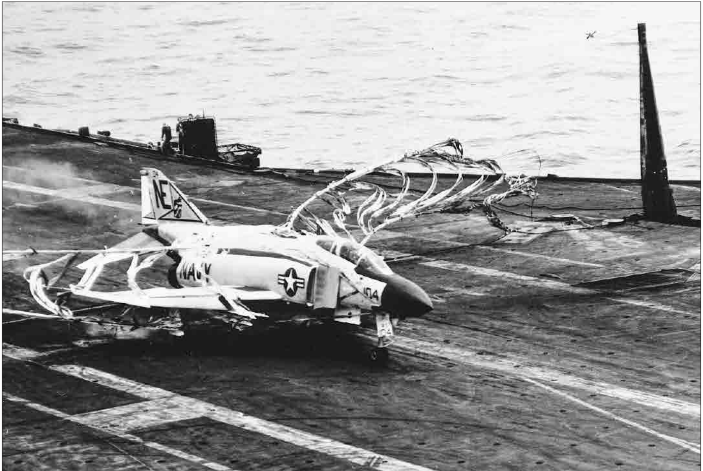
An F-4J Phantom II, BuNo 155752, of VF-21 slams into the barricade on board Ranger (CVA 61) during Carrier Air Wing 2's Vietnam War operations between 14 October 1969 and 1 June 1970. Both crewmen were uninjured and the aircraft received minimal damage.
