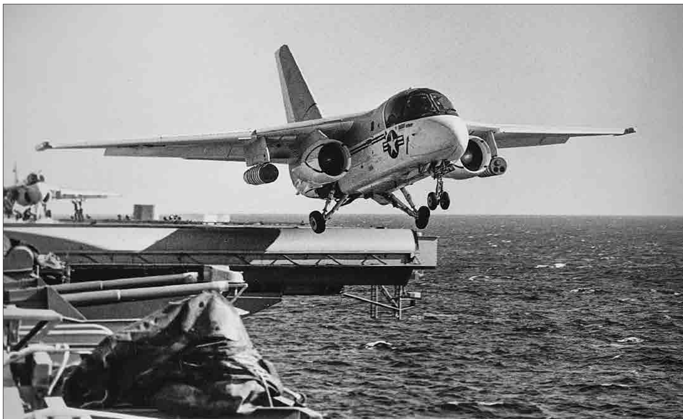
An S-3A catapults from Forrestal (CVA 59) during the Viking's initial carrier suitability tests.
