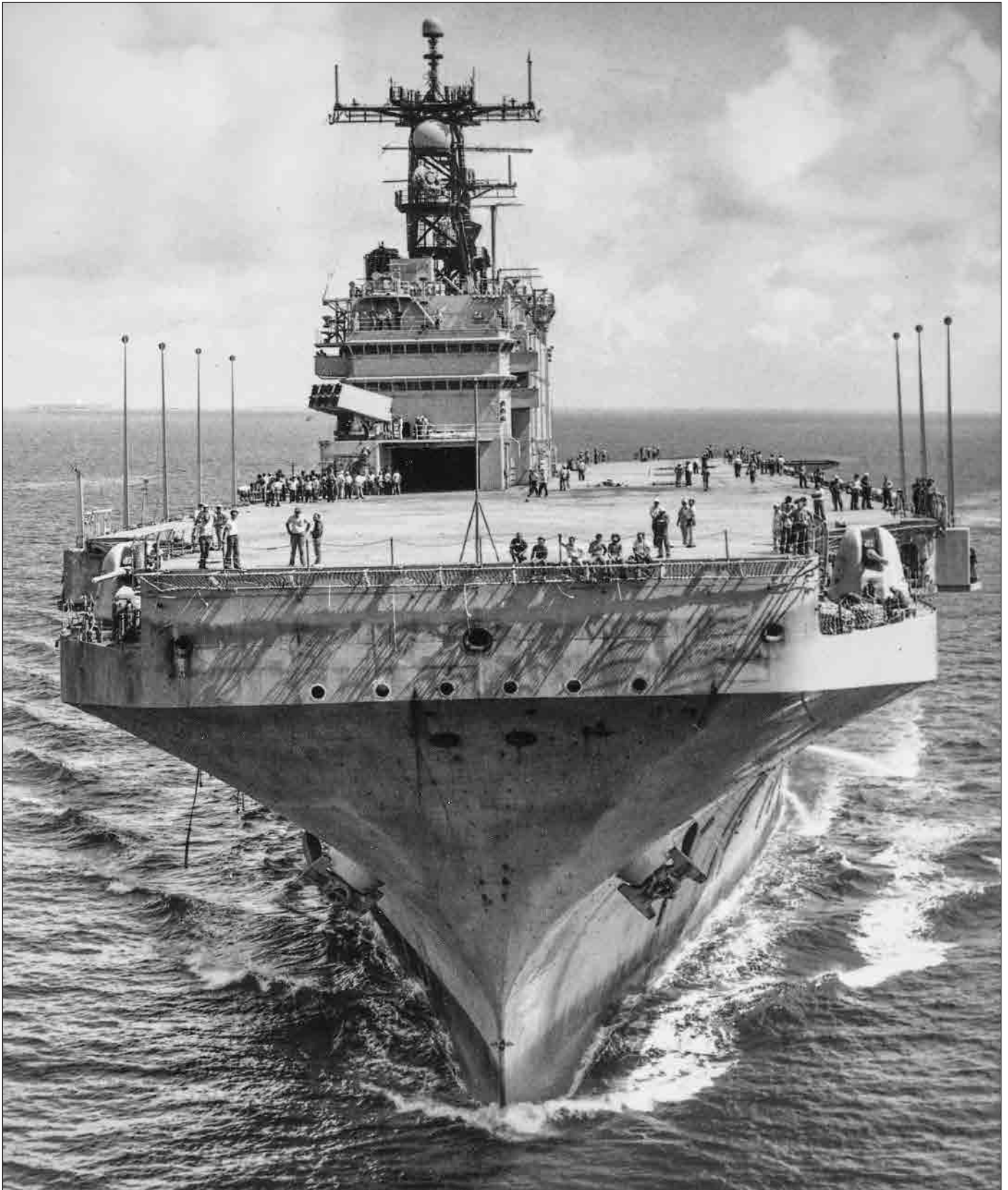
Tarawa (LHA 1) is the first of a new class of five amphibious assault ships. These combined in one ship type the functions previously performed by four different types: the amphibious assault ship (LPH), amphibious transport dock (LPD), amphibious cargo ship (LKA), and dock landing ship (LSD).
