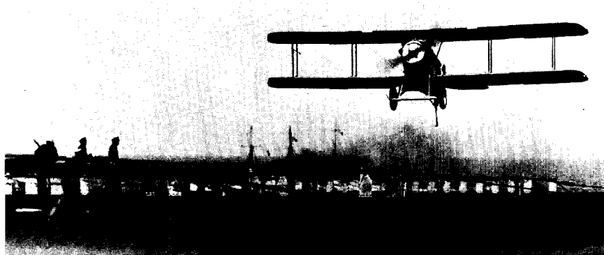
A VE-7 AIRCRAFT lands on USS Langley in May 1927, using longitudinal wires on fiddle bridges for an arresting arrangement. Note tail hook on plane and masts of sailing ship under wings.
