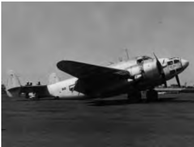
The squadron's first aircraft was the PV-1. This photo shows a PV-1 at San Juan, P.R., with a collapsed tail wheel, 21 March 1944, 80-G-411758 (Courtesy Captain Jerry Mason, USN).
