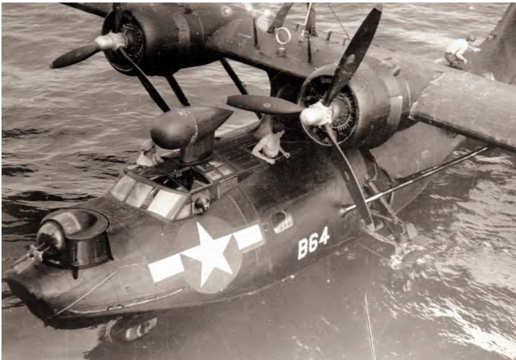
A squadron PBY-5A coming up the launching ramp (Courtesy Fred C. Dickey, Jr. Collection).
