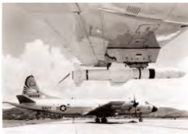
A close up of a Harpoon missile on the pylon of a squadron P-3. A squadron P-3C is in the background.
