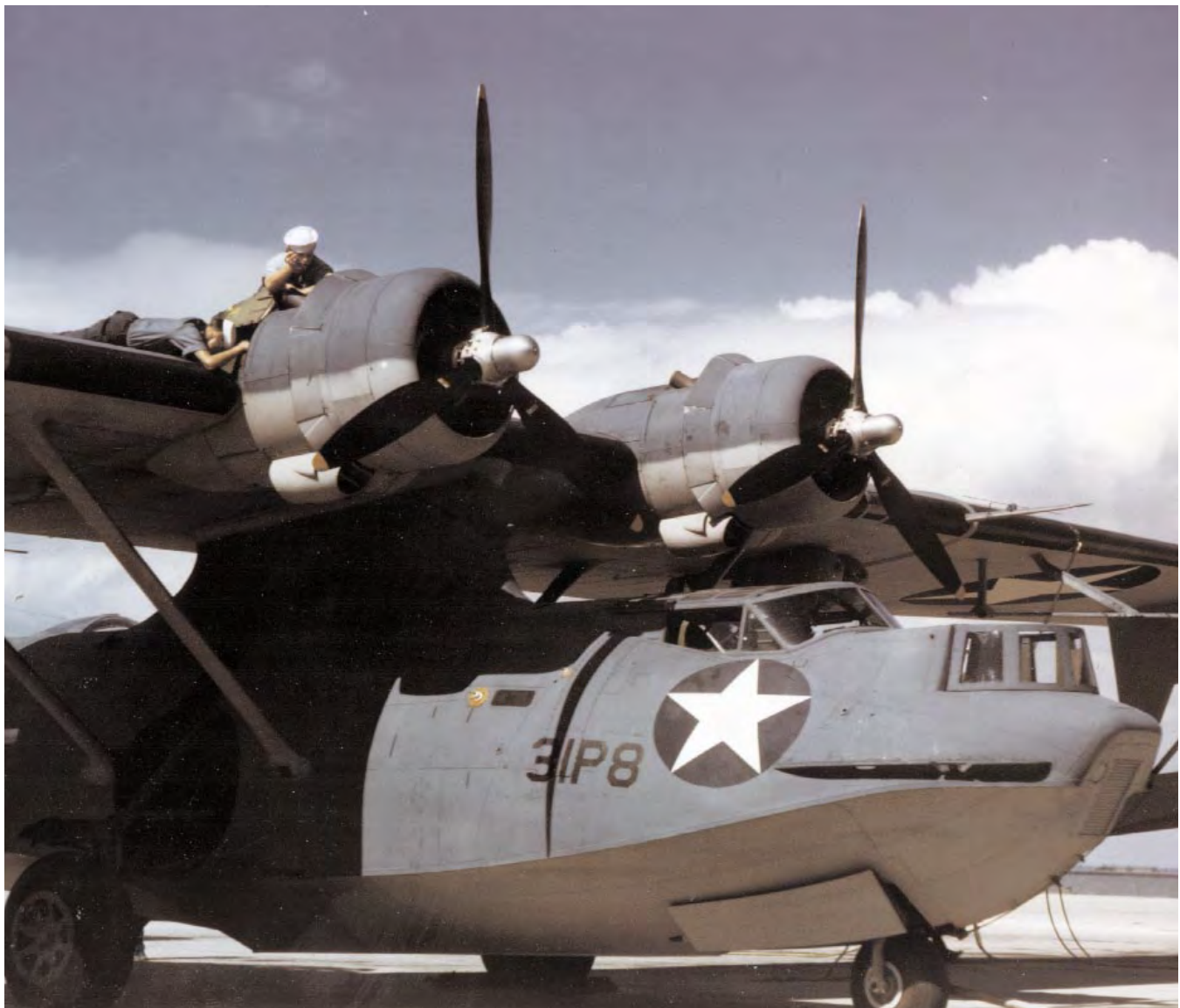
Squadron aviation machinist's mates work on the starboard engine of their PBY-5A, circa 1942, 80-G-K-15310.
