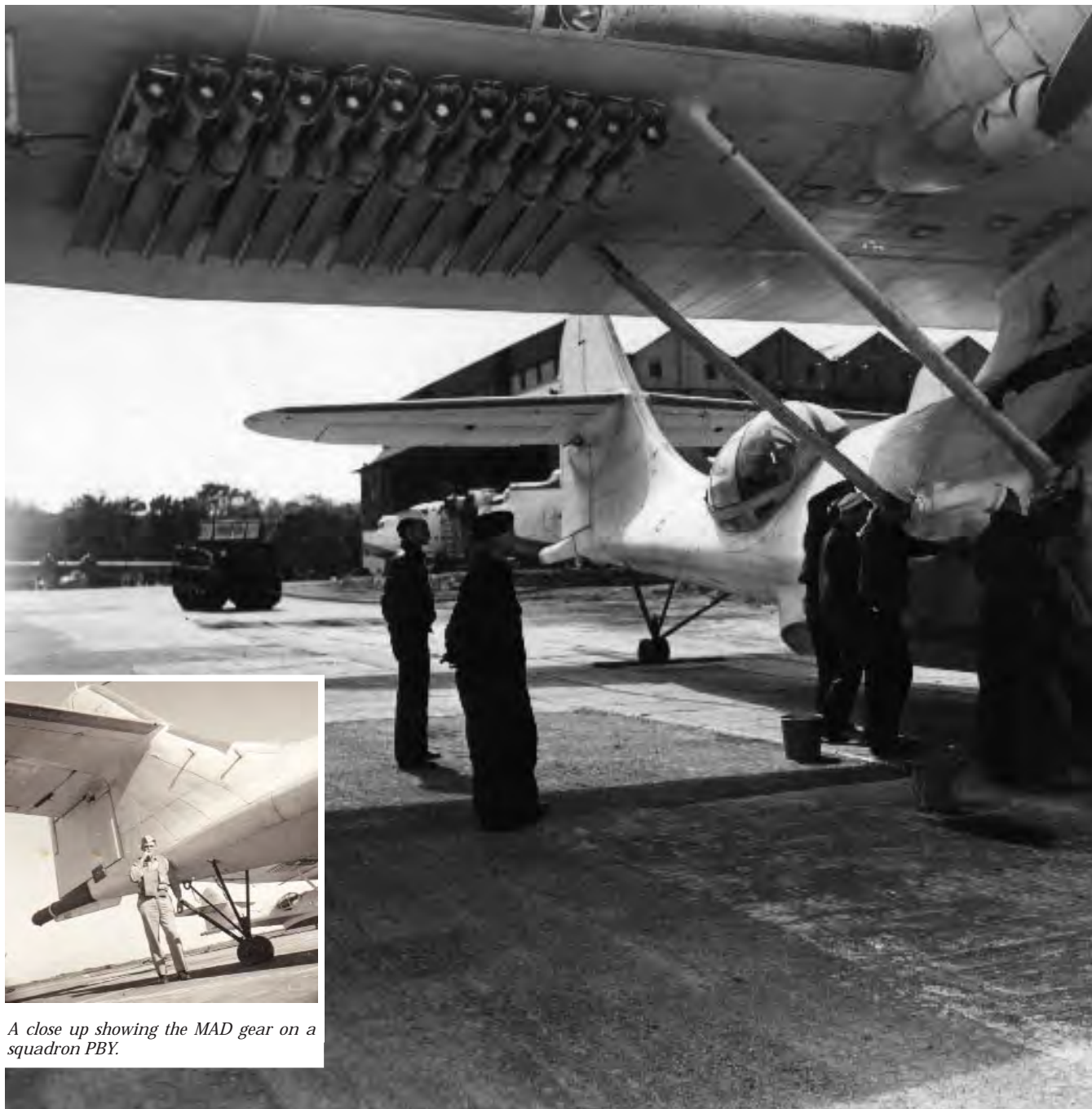
A close up of a squadron PBY-5A showing the rails on the wing for retrorockets, 80-G-53255 (Courtesy Captain Jerry Mason, USN).
