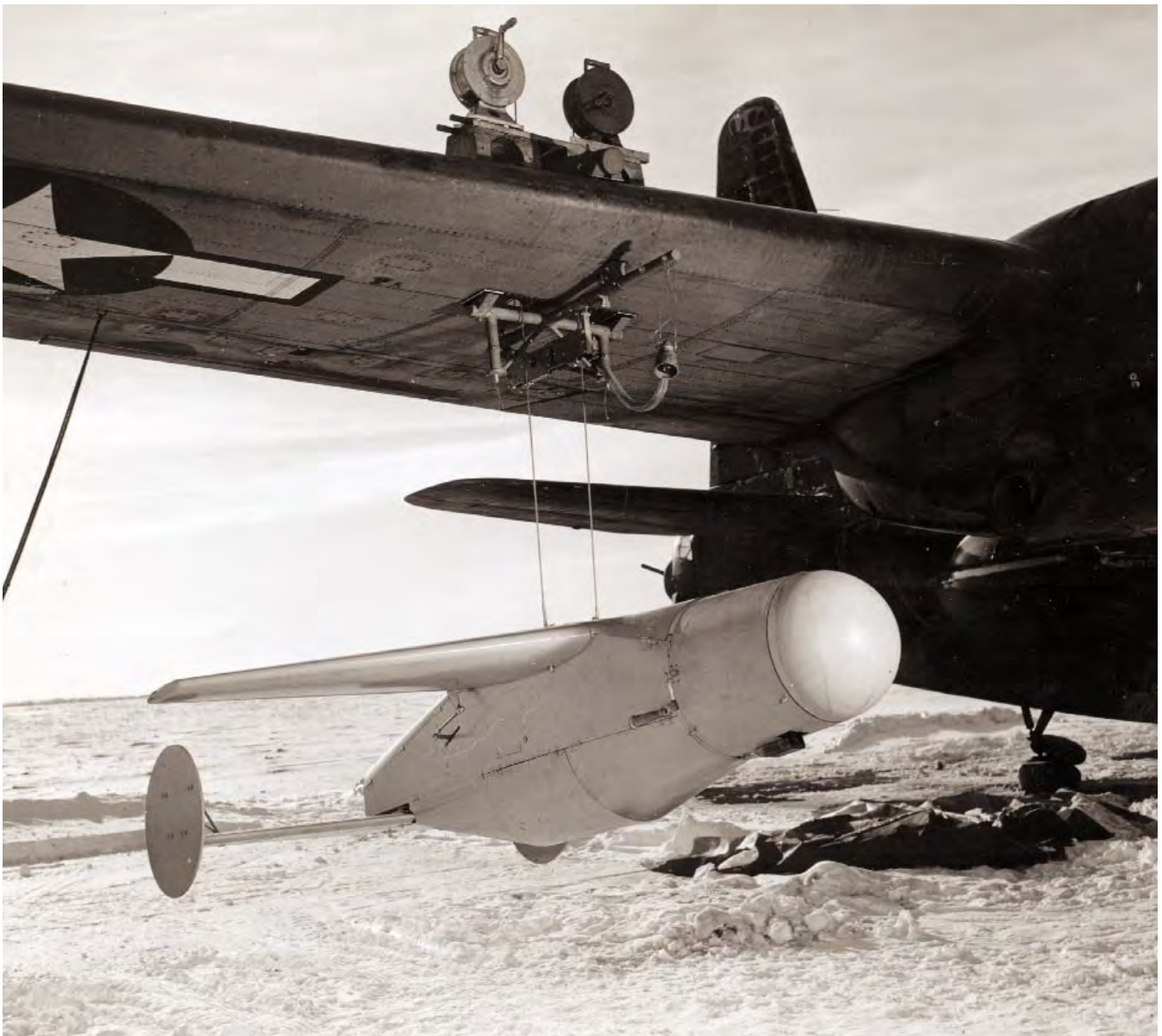
The squadron used Bat missiles in the Pacific during the latter part of the war. This photo shows a Bat missile being placed in position on a PB4Y.
