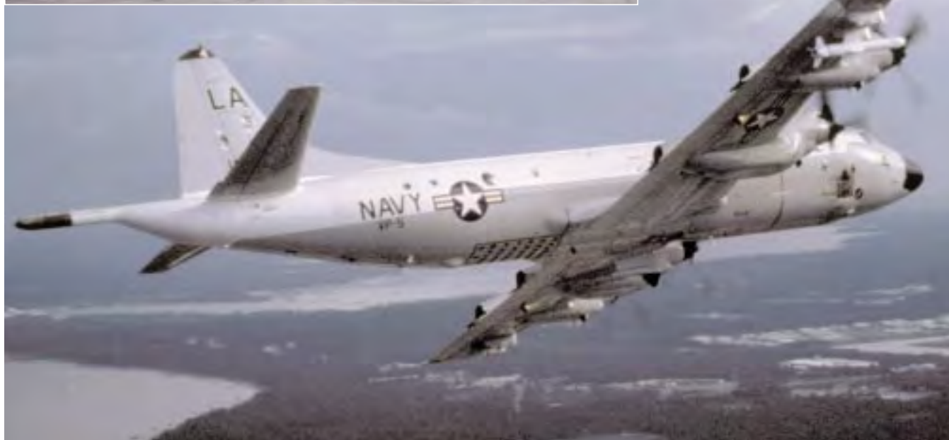
A squadron P-3 Orion in flight with a Harpoon missile under the wing.
