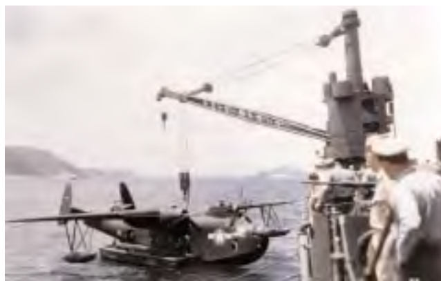
A squadron PBM-5 being prepared for lifting aboard a seaplane tender, Kerama Retto anchorage, Ryukyu Islands, circa April-July 1945, 80-G-K-14006.
