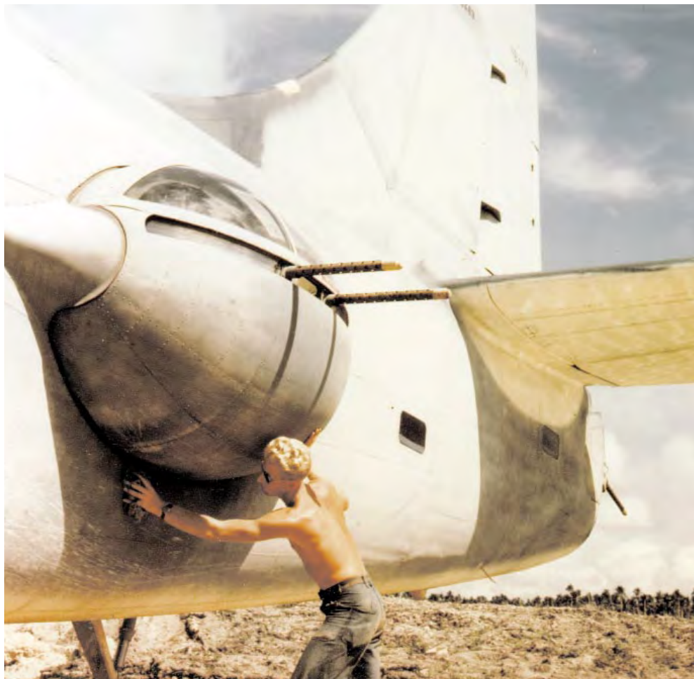
A close up of the port waist twin .50 caliber machine gun on a PB4Y, 80-G-K-14546.
