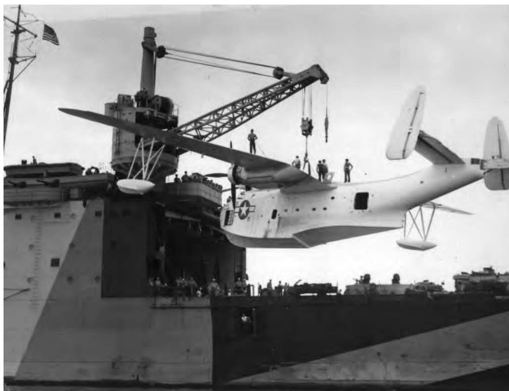
A squadron PBM-3 being hoisted aboard Albemarle (AV 5) at Guantanamo Bay, 5 January 1945, 80-G-304428 (Courtesy Captain Jerry Mason, USN).
