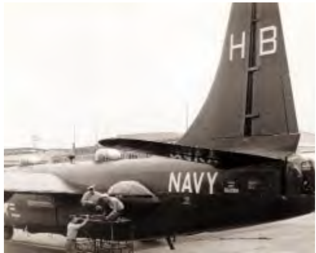
A close up of a squadron P4Y-2 showing personnel installing a .50 caliber machine gun in a side turret, 1952.
