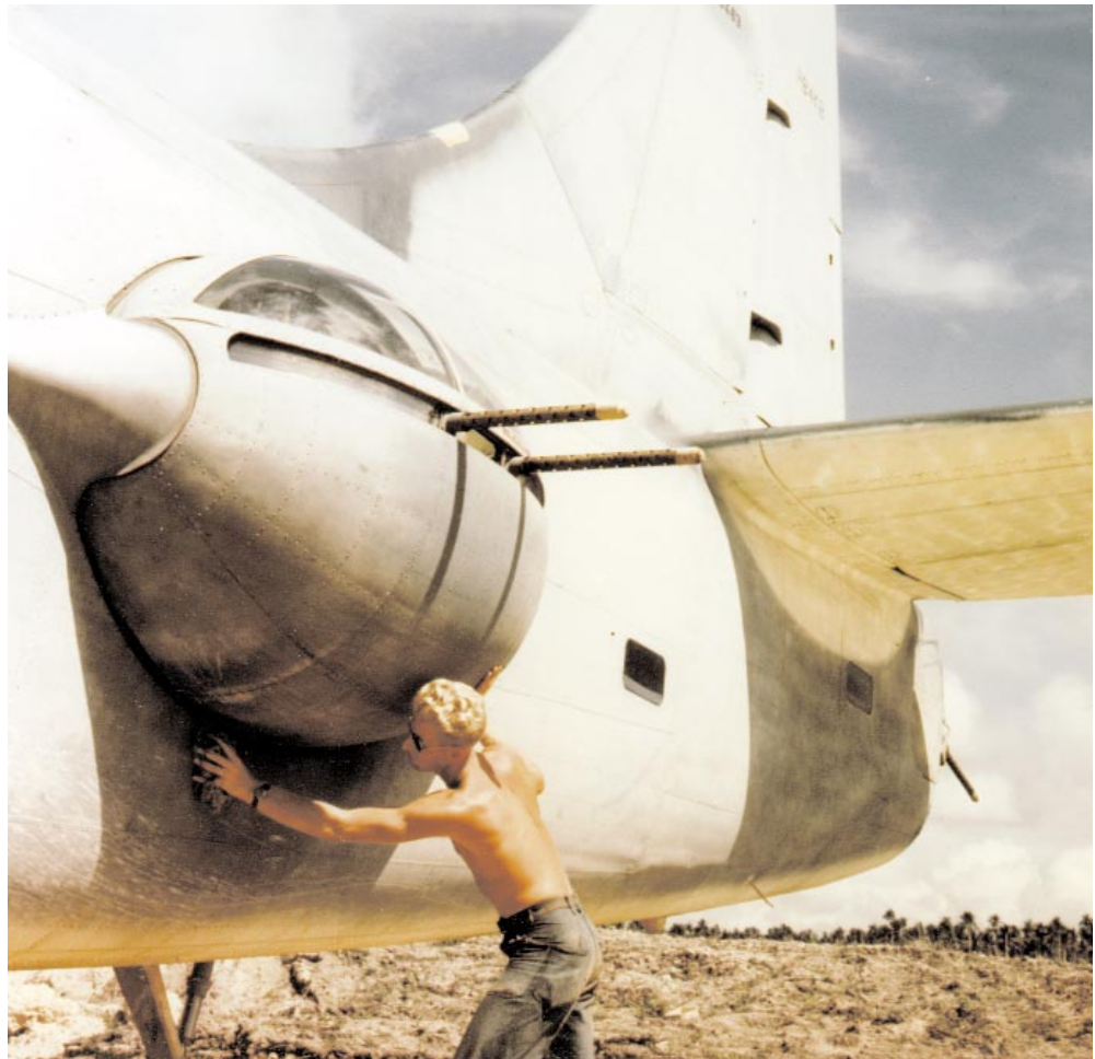
A close up of the port waist twin .50 caliber machine gun on a PB4Y, 80-G-K-14546.
