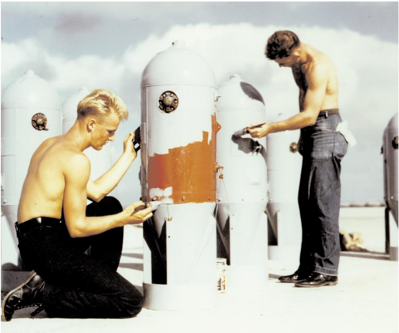
Aircraft depth bombs receive a fresh coat of paint from aviation ordnancemen, 80-G-K-15110.
