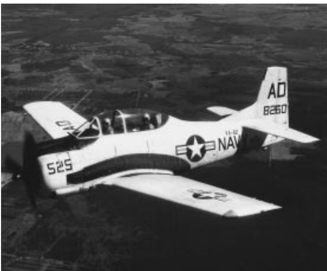
A T-28B Trojan used by the squadron for instrument all-weather flight training.
