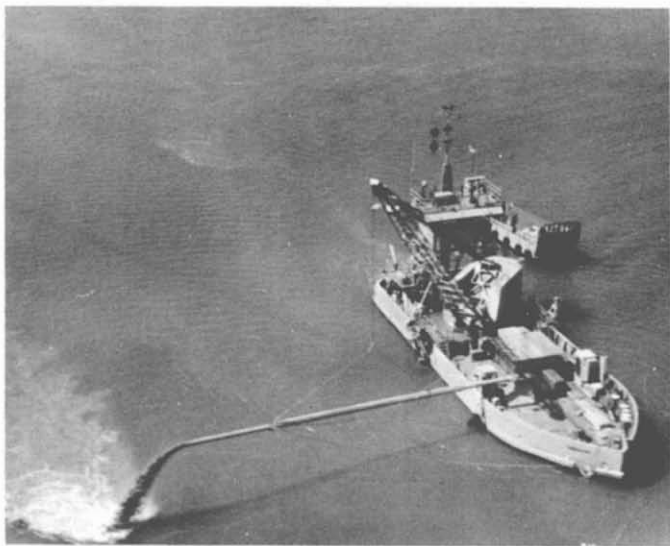
34. Sidcaster Dredge: SANDCASTER. The 12-inch sidcaster dredge SANDCASTER removes shoals on the Cua Viet River—less than 5 miles from the DMZ.
