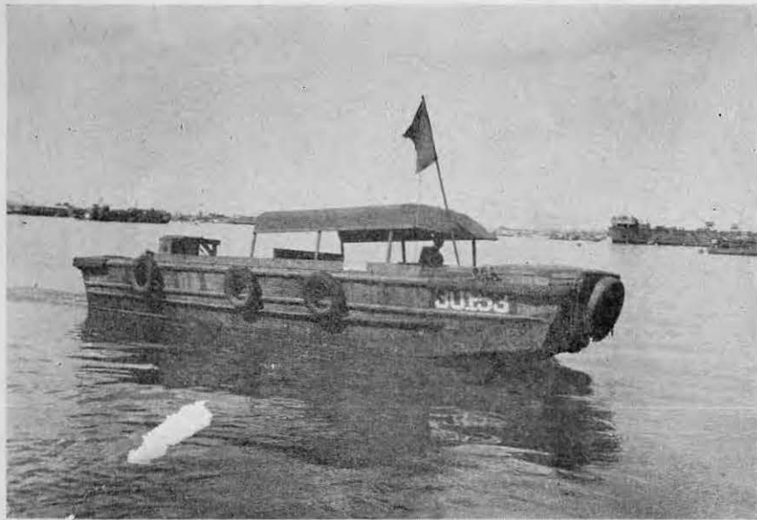
The Powder Control boat used to detonate the underwater charges
