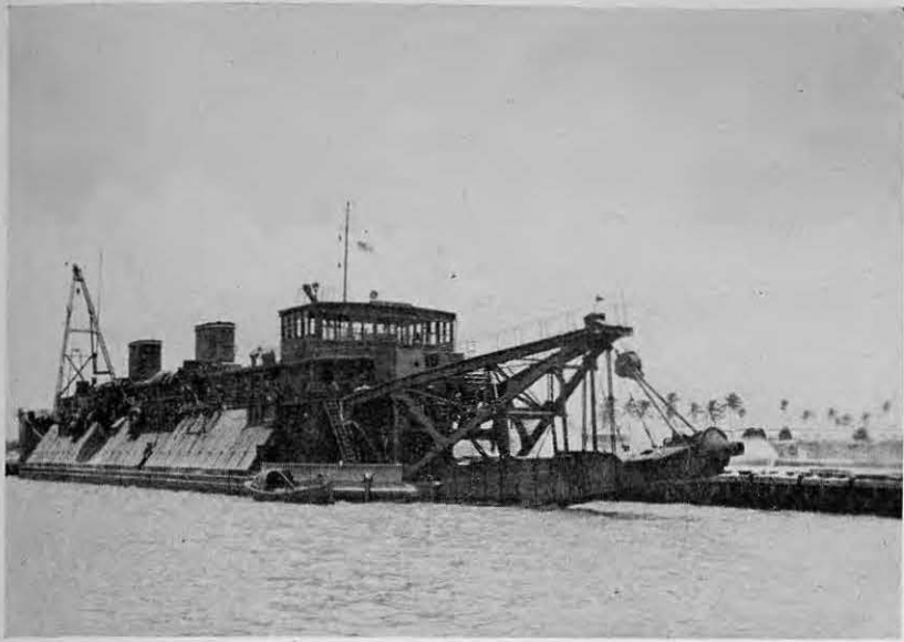
Dredge YM-21 at Guam, still wearing her sheathing put on for the long tow from the Great Lakes to the Marianas
