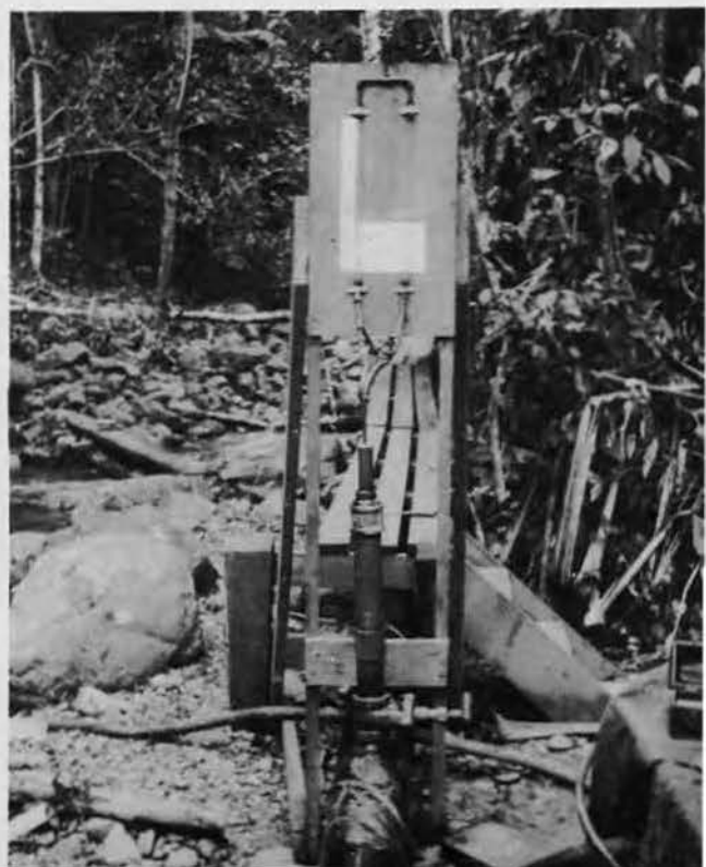
Below: Improved pitometer installed on line from Nubai Creek at Hollandia. This mechanism was designed and built by Lt. Spalding, Chief Burke, with intricate machine work performed by Walter Kant. Pitometer measured amount of water being supplied through Naval Base system, which reached peak of 960 gals. per minute. Glass tubing on board registers differential between pressure head and velocity head.
