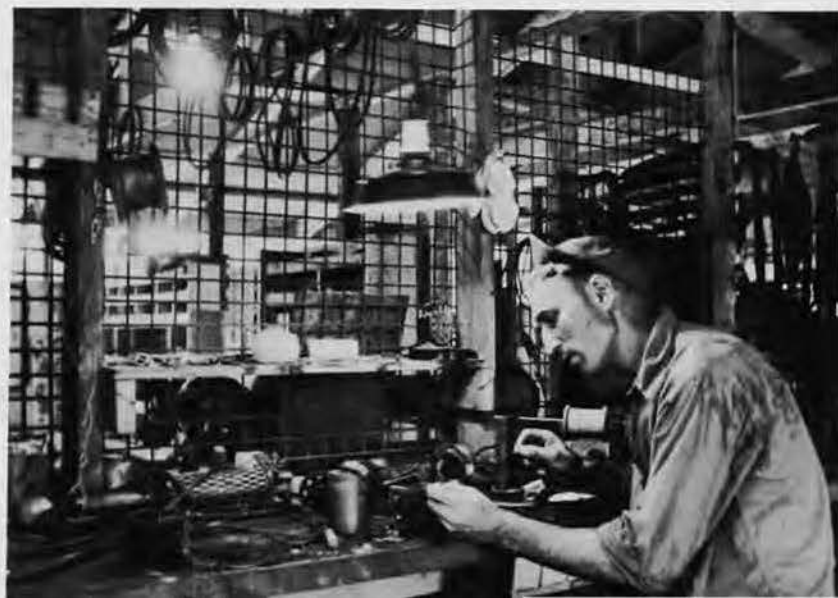
Expert on electric motors, Anthony Kelt winds an armature.
