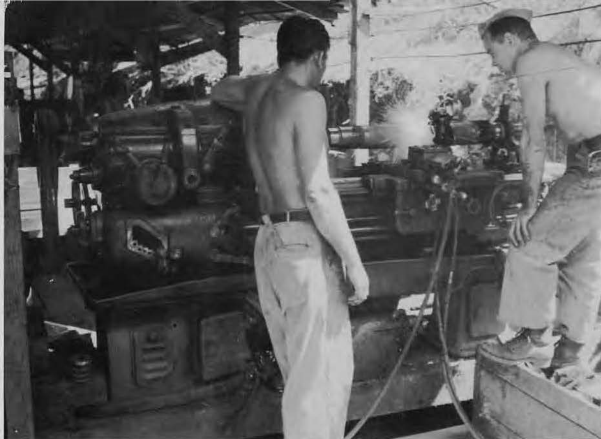
Machinist Walter Kant, left, explains the intricacies of the metalizing process used in building up a shovel drum shaft to Chief M. T. Bryant.
